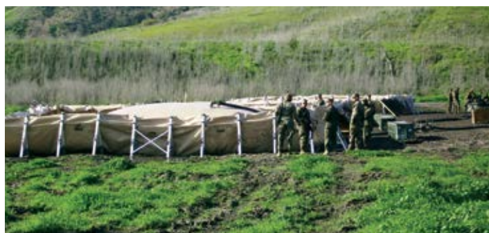
Military field application containing a flexible fuel tank—deployed in 45 minutes by five people.
